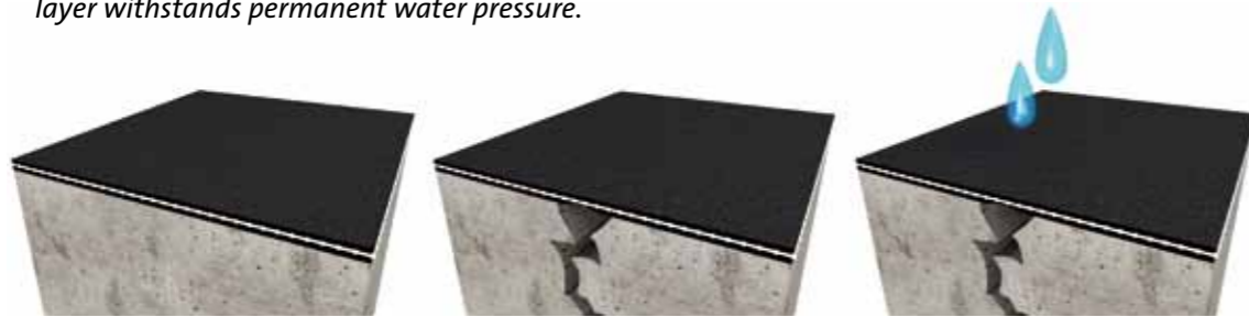
3. Crack bridging due to an embedded mesh. The mesh separates the top waterproofing layer from the crack and helps significantly to withstand permanent water pressure.
